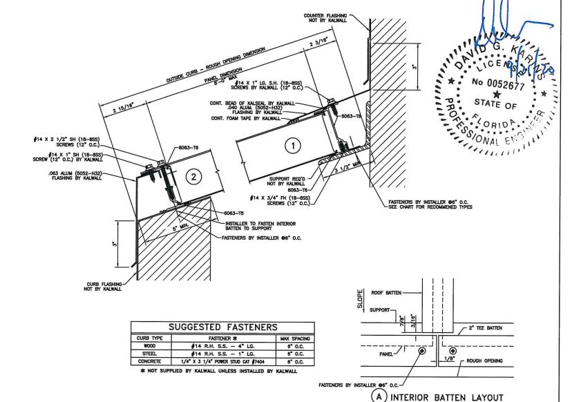
INSTALLER TO SET ENTIRE PERIMETER EDGE IN A CONTINUOUS BED OF CAULKING, AND ISOLATE ALUMINUM FROM DISSIMILAR METALS TO PREVENT ELECTROLYSIS.
